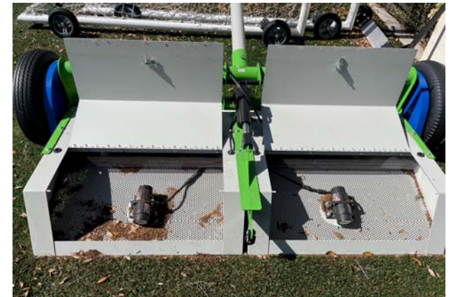
Dual Vibrating Motors (no infill displacement)
