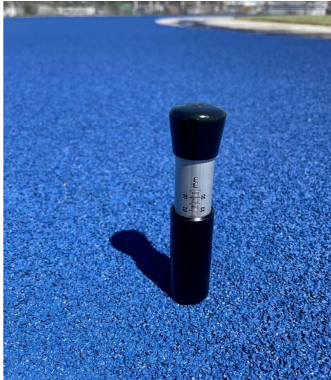
Surface Depth Gauge Testing (13 mm min.)
