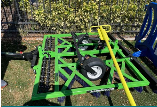
Turf Groomer (level infill and decompact)
