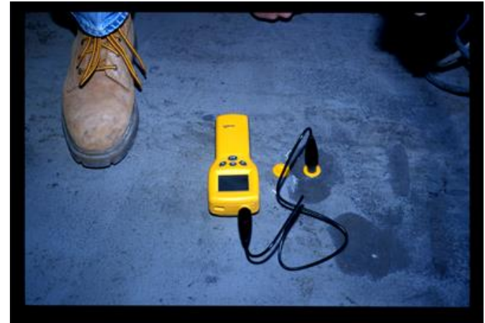
Moisture Test Kit in Use ASTM F-2170-11 (RH Probe)
