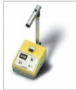
Readings from the Roof Moisture Gauge are taken & recorded at each grid point.
