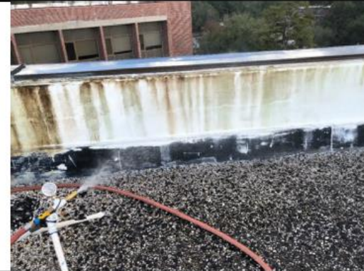
Photo 16: General photo to show position of hand-held nozzle directed at parapet. See Photo 17 for pressure at gauge.
