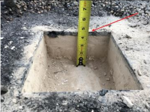
Photo 31: Core #4 was approximately 4 ½ inches in depth. Note the core location shows no evidence of moisture. Core samples #3 and #4 were approximately 19 feet apart. This indicates a slope of approximately 1 inch within 20 feet.
