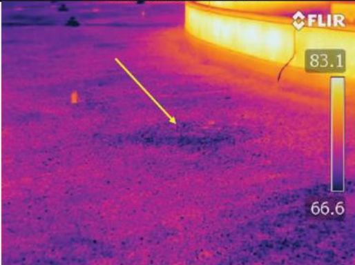
Photo 32: IR image of Core #3 showing thermal anomalies consistent with findings at time of the core sample.
