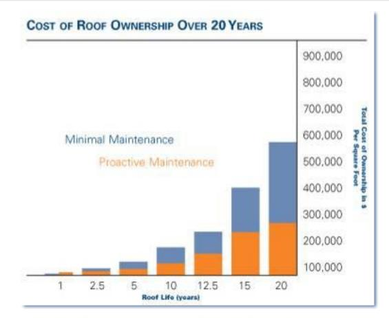
Based on 100,000 SF roof; Original cost \$350,00 Tear-off and replacement cost \$500,00; Leak repairs \$750 per occurrence. PM costs: Annual inspections - \$1000; Annual Visual Surveys \$1000; Periodic moisture scans \$5,000
